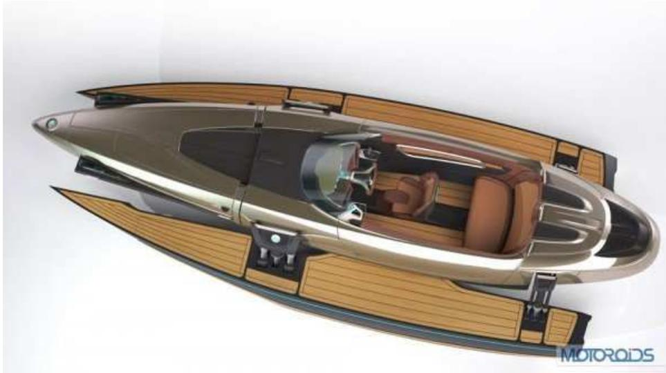
*Kormaran in trimaran mode has three separate hulls for added stability.*
