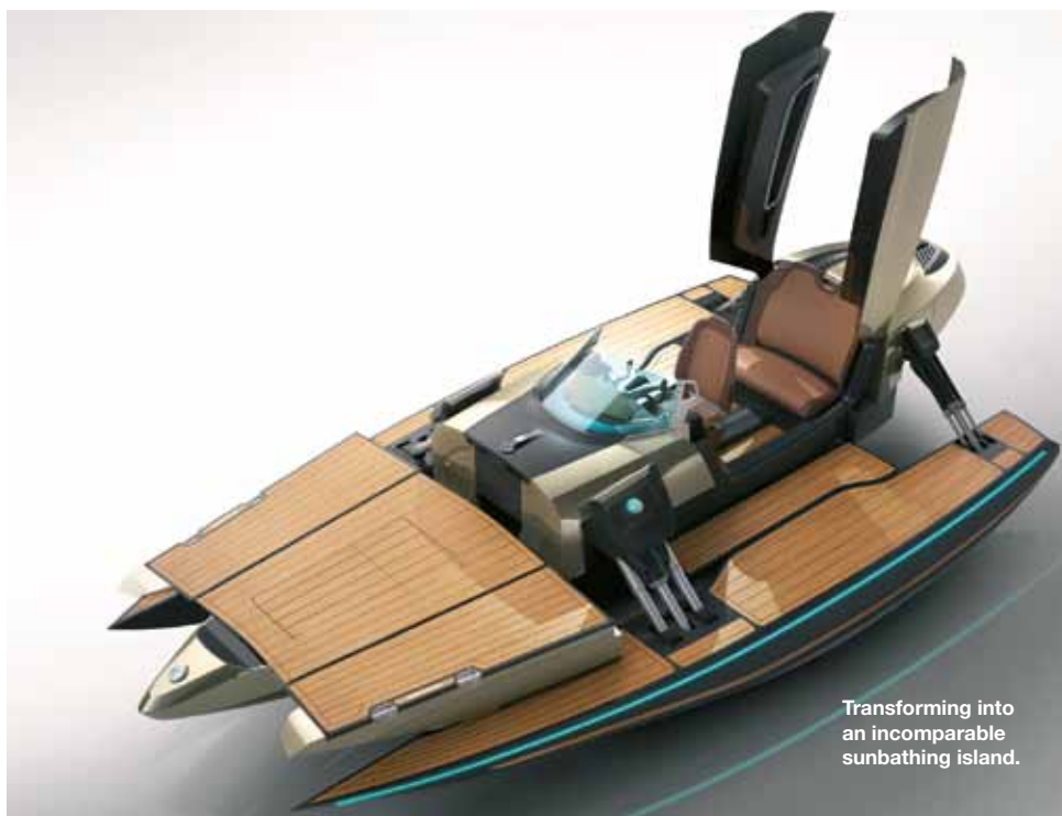
The Kormaran combines the agility of a monohull with the stability of a catamaran or trimaran.
